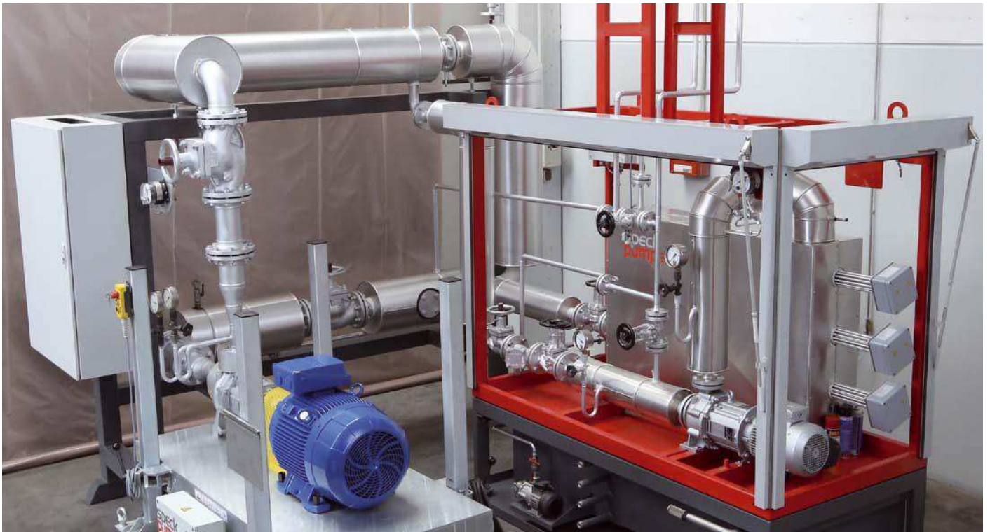
Thermal oil test stand with pump surveillance system on the premises of Speck in Roth.
